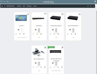
Select the remote icon on the Cisco Telepresence tile. The button builder will be opened and additional buttons with extra commands and/or macros can be added.
