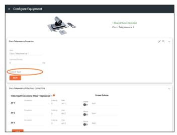
18. Select SSH, Telnet, or RS232 from the Control Type drop down. New information fields will open.
